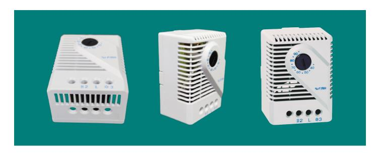
The HS01 is a device specifically designed to regulate the relative air humidity within enclosures. Its main purpose is to prevent condensation and corrosion, which can lead to damage and malfunction of electronic components. By connecting the HS01 to an enclosure heater, also known as a dehumidifier, it can effectively raise the dew point within the enclosure.
